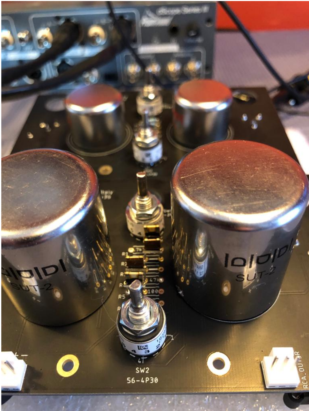
Fig. 1 SUT2 board and SUT3 board compared while at the test bench for final quality acceptance: SUT2, front board, is noticeably larger and the Z foils resistors can be spotted between the greyhill switches.
